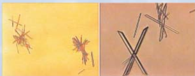
Electron microscopy of calcium sulfate (CaSO 4 ) scaling crystal
